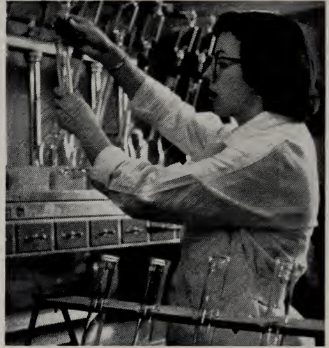
An Illinois technician determines the protein content of a food by the Kjeldahl method.
